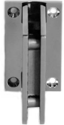
#85.112 ; 90 degree angle glass hinge on plate; for 10 to 12 mm -3/8 to 1/2 inch glass; leaf: 89 x 58 mm; (3 1/2 x 2 1/4 inch) Plate: 90 x 49.5 mm (3 1/2 x 1 15/16 inch)
