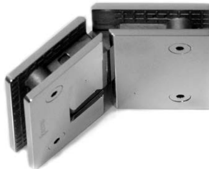
#85.109 ; 135 degree glass hinge for 10 to 12 mm -3/8 to 1/2 inch glass; leaf: 89 x 61 x 65 mm; (3 1/2 x 2 3/8 x 2 1/2 inch)
